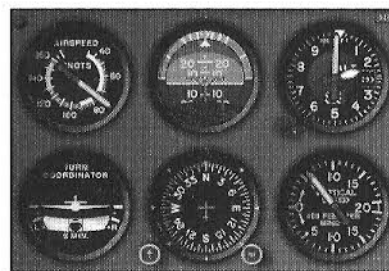
Figure 1.12 The Turn: the airspeed is lower than normal cruise; the heading indicator shows a left turn, and the turn coordinator shows a balanced, standard-rate turn; altitude indicator is constant.
