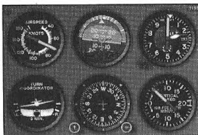
Figure 1.15 The Climbing Turn: the climb airspeed is steady; the attitude indicator shows 8° of bank, climb attitude; the heading indicator shows a left turn; the turn coordinator shows a half standard-rate, balanced turn; altitude is increasing as shown by the altimeter and vertical speed indicator.
