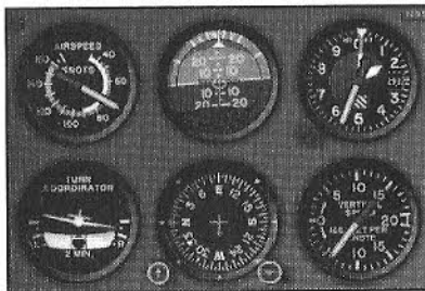
Figure 1.15 The Climbing Turn: the climb airspeed is steady; the attitude indicator shows 8° of bank, climb attitude; the heading indicator shows a left turn; the turn coordinator shows a half standard-rate, balanced turn; altitude is increasing as shown by the altimeter and vertical speed indicator.
