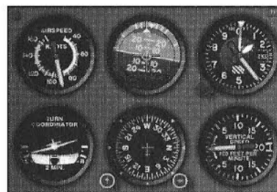
Figure 1.12 The Turn: the airspeed is lower than normal cruise; the heading indicator shows a left turn, and the turn coordinator shows a balanced, standard-rate turn; altitude indicator is constant.
