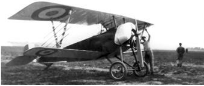
A Nieuport Scout with rocket rails on its struts. The rockets were fired electronically from the cockpit against targets such as observation balloons. (Courtesy Smithsonian Institution)
