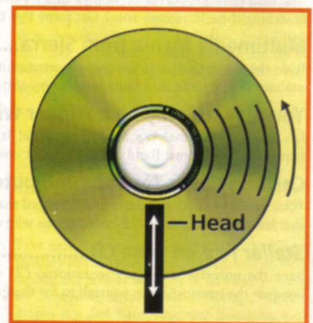
Laser lenses scan the surface of a CD, looking for the right information.
